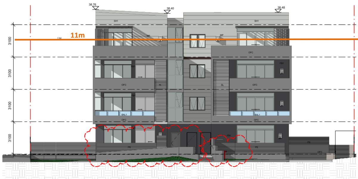
Figure 16: Extract of Southern, front elevation showing areas of non-compliance
